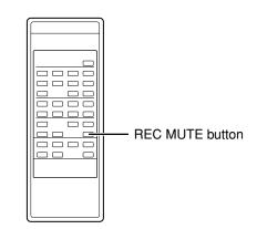
The display will indicate "Rec Mute" and muted recording will begin. After approximately four seconds, the recorder will enter record-ready mode.
